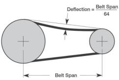
• Check fan and motor shafts for parallel and angular alignment. Make sure motor and fan sheaves are aligned properly and if needed use a straight edge to align the sheaves properly.
