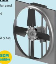
Available in sizes 10" through 54" with aluminum or glass reinforced polypropylene blades, these fans are manufactured for durability and economy. The all welded pipe frame motor support will accommodate a wide range of motor types. Capacities range from 300 to 39,000 CFM and up to 1.25" static pressure.
