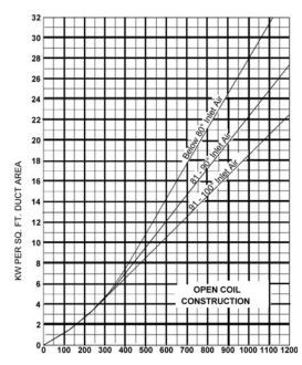
Fig. 5 – MINIMUM AIR VELOCITY REQUIRED (FEET PER MINUTE)
