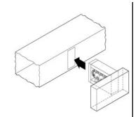
Fig. 2 - Installation drawing of slip-in heater.
