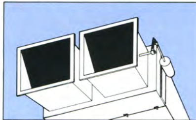
MHV7B and MHV8B Dual Duct Mechanical Reset Constant Volume with temperature proportioning inlet valve. Two motors.
