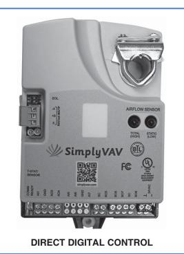
Every SimplyVAV purchase will require at least one digital thermostat. This is used for setup, commissioning and balancing of the controller/actuator, and it allows you to assign an address, or name, to each VAV, so that they are easily distinguishable by a BACnet<sup>®</sup> System. There is a QR code sticker on each thermostat, which takes you to a website which will walk you through setup and calibration. It's an on board installation manual.
