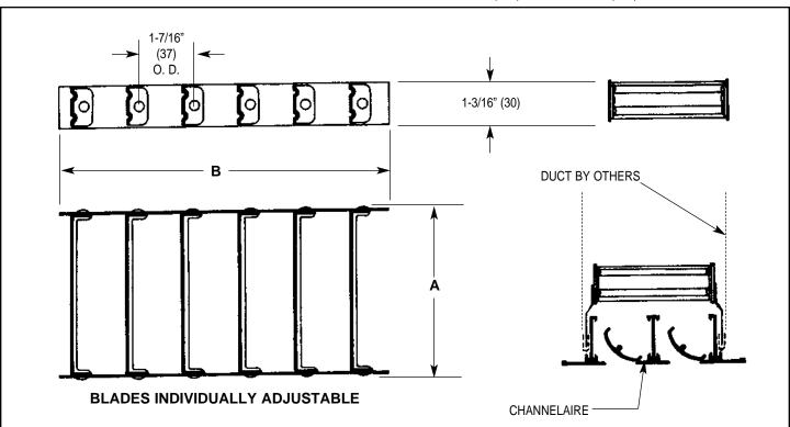
Model CXEA deflector will be received with tabs folded over. Unfold tab and insert deflector into hemmed portion of duct. Deflector must be sized so "B" is 4" (102) shorter than length of manufactured sections of Channelaire.
