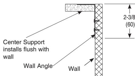
Center Support Mounted flush with wall (Shown aligned horizontally).
