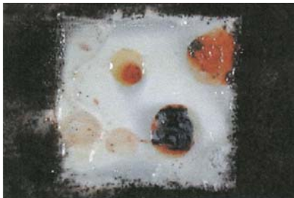
Fungal Growth Rust Formation
