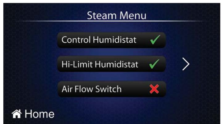
A Red “X” will be displayed to indicate if the control is not sending a signal. If any one component is not satisfied, the “Home Screen” will display an indicator when one or more controls are not satisfied. The Steam Output number and the “Steam” menu icon will illuminate in “RED”.
