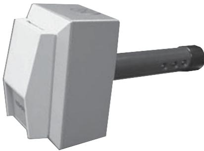
The Model HXHAN is an intelligent humidistat solution used exclusively for duct mounted installations. The humidistat is capable of providing both humidity and temperature measurements from inside the duct. The microprocessor control takes the temperature into consideration when calculating the humidity to provide an extra degree of precision.
