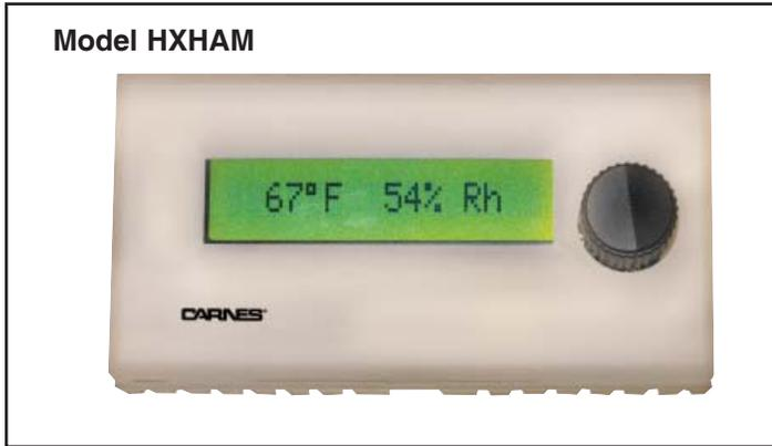
The Model HXHAM is a wall-mounted, microprocessor-controlled humidistat solution for cutting edge humidity control. The HXHAM employs a backlit LCD module, which displays both the ambient temperature and humidity of the surrounding air. The embedded software allows user navigation between temperature/humidity viewing mode and setpoint adjustment mode, and also outdoor temperature and humidity viewing mode.
