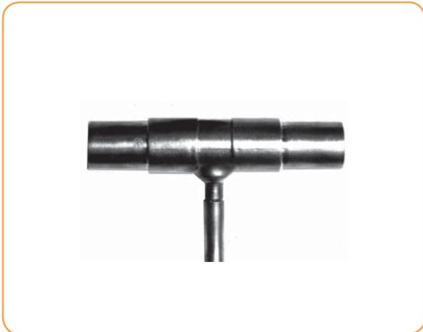
Steam hose drain "T" are available for use when the duct is located below the top of the humidifier or where the length of steam hose is in excess of 12 feet.
