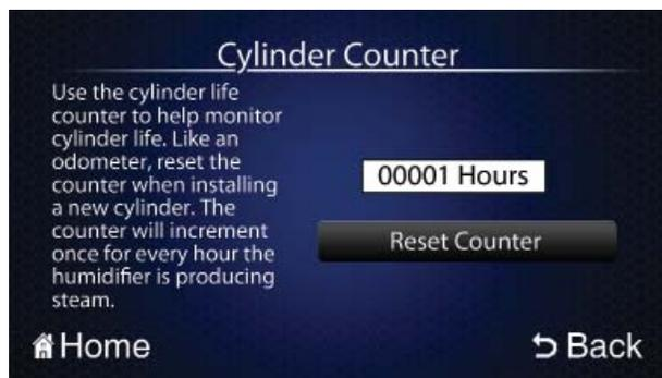
This page consists of a counter where the user can monitor the life, in hours, of the cylinder. When changing a cylinder, press the ‘Reset’ button on this page to reset the timer. The Cylinder Life Counter only counts the amount of actual runtime of the cylinder (the time when the contactor is pulled in). The counter value is saved even when the humidifier is powered down. The national average
