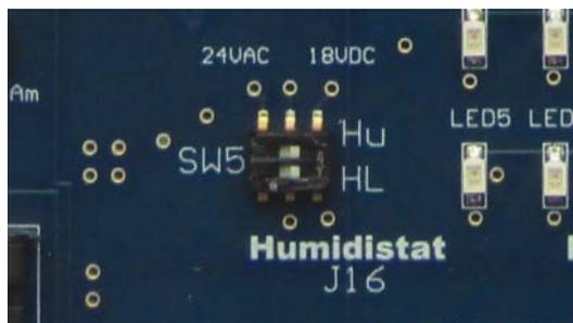
Two cylinder humidifiers may be wired for simultaneous or separate and independent operation. Controls should be connected to the terminals on the circuit board as shown below using No. 20 AWG wire. Attempting to use two wires in a single control connection will require a No. 22 AWG wire or less. See wiring diagram for parallel connections. Avoid running control wiring near high voltage primary wires due to the possibility of interference and signal distortion.
