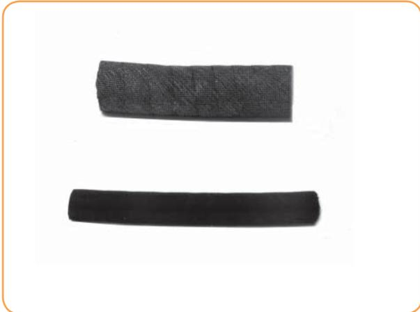
Carnes steam hose is made from EPDM compound to withstand the low pressure steam without deterioration. Model HXSAB steam hose has an I. D. of 7/8" for use with units that use "AX" or "B" steam cylinders. Model HXSAC has an I. D. of 1-5/8" for use with units that use "C" cylinders. The hose may be easily cut to the exact length at time of installation.
