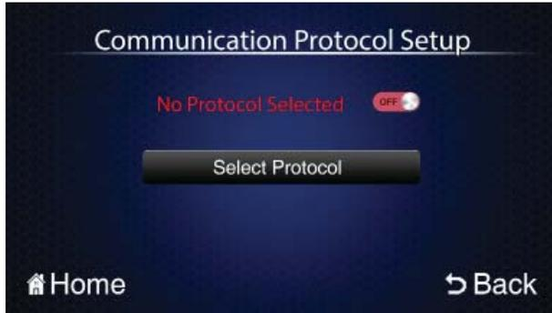
This page is where you can select and setup the communication protocol you will be using with your Building Management System (BMS) for full external monitoring capabilities. (See the CarnesLink Communication Protocol Installation, Operation and Maintenance Manual for further information.)
