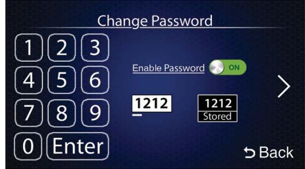
This page is where the password for the settings menu can be changed or disabled. If the password for the Settings menu is forgotten the it can be reset. To do this, remove power to the humidifier, flip the switch SW3's bottom “Clear” switch to the right and power the unit back on. Return the switch's afterwards from the right to the left.
