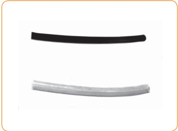
Two models of condensate return line are available. Model HXRA has an I. D. of 3/8" and is used whenever steam distributor pipes are used with the humidifier. Model HXLA has an I. D. of 5/8" and is used with optional fan distribution units.
