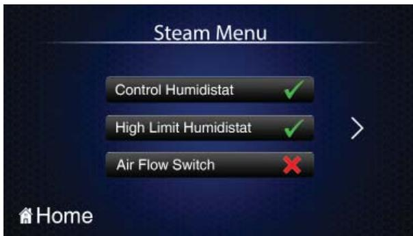
The “Steam Menu” page will display the status of the four basic controls (Control Humidistat, High Limit Humidistat, Air Flow Switch, and Door Interlock). The humidifier will only produce steam when the unit is switched into the “ON” position and if all four controls are satisfied.
