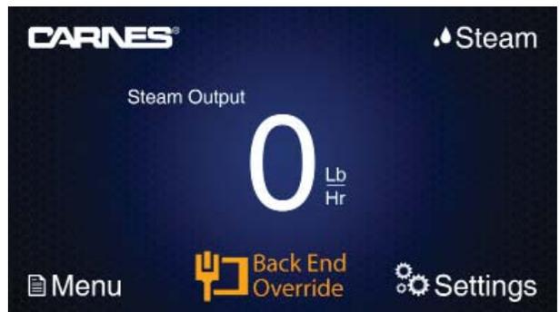
When CarnesLink is being used, the “Back End Override” indicator is displayed only when the connected building management system requests the unit to be set to “off” or “drain” while the unit is “on”. When selected more information is provided about the override.
