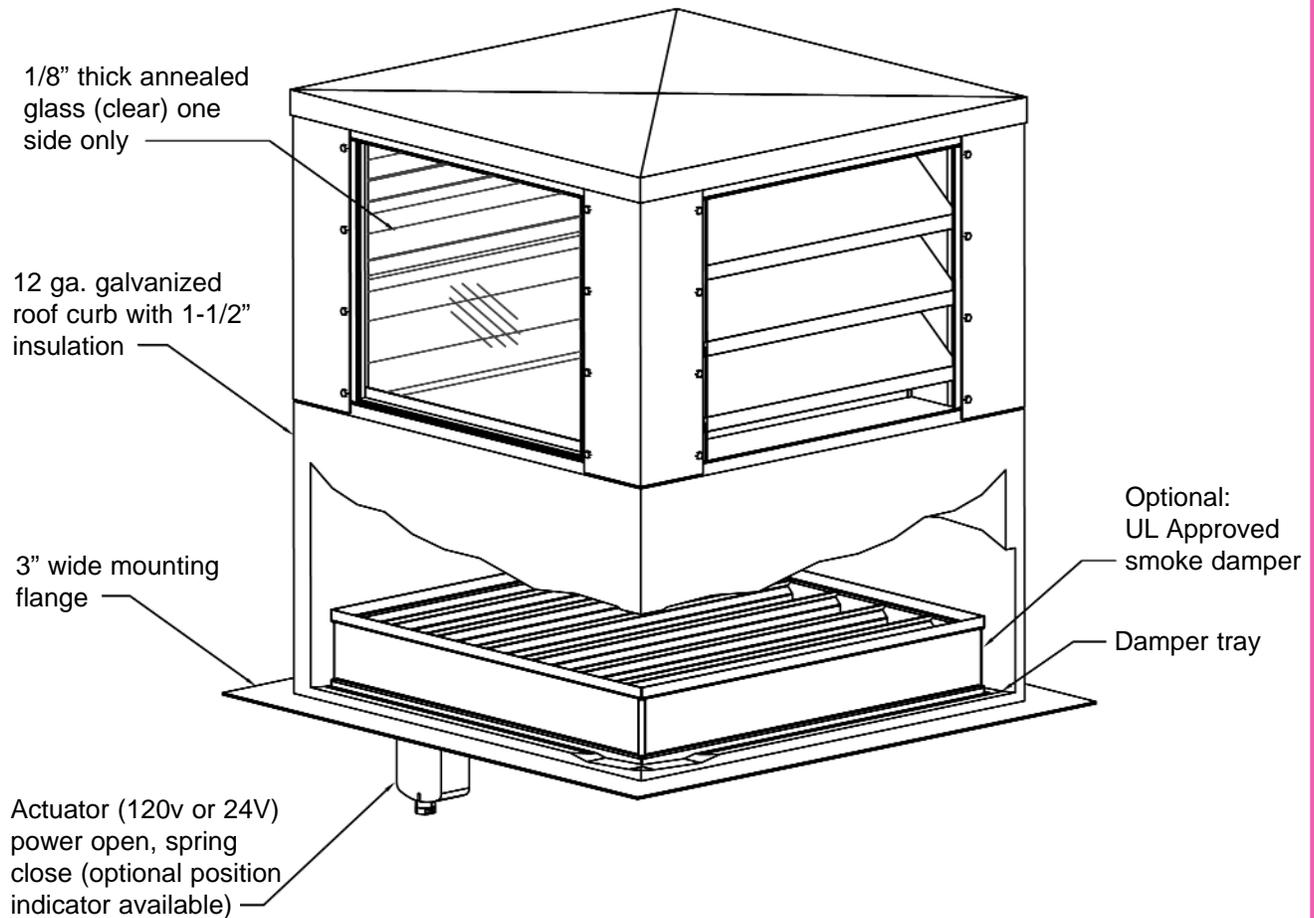
The Carnes Company is pleased to announce our newest product addition - the PEAB louvered penthouse elevator vent assembly. Designed with three louvered sides and one side of 1/8" annealed glass, the PEAB assembly is built specifically for ventilation and emergency smoke evacuation of elevator shafts.
