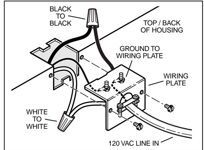
Ventilator can be wired from outside of housing.
