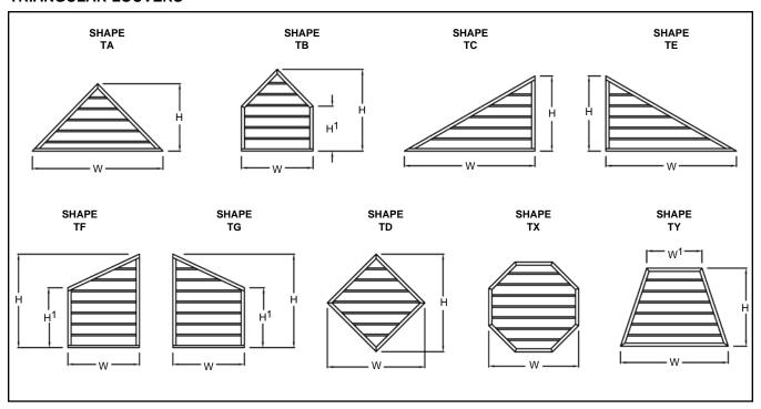
Note: Special shaped louvers are not AMCA tested for water penetration or air flow resistance. Conservative air flows should be used when sizing louvers to help prevent water carry over.
